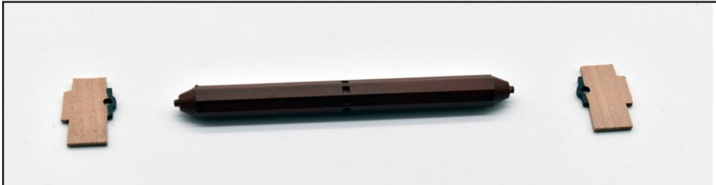
91. Main Windlass. For Sherbourne, this is a very simple assembly consisting of just three parts - the sides (83 - left and 84 - right). Paint the cap squares of the winch sides black, and the winch itself a dull red or wood colour.
