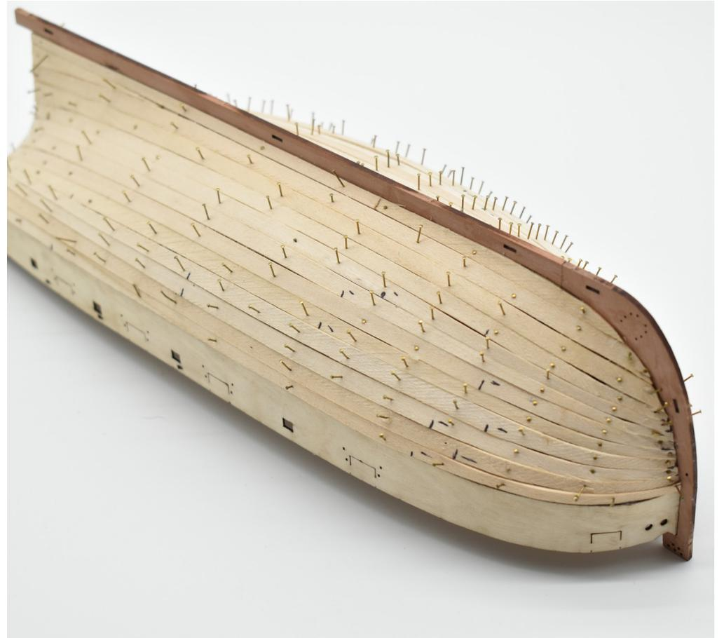
32. Once the planking is complete, remove every single pin from each of the planks. The hull can be sanded smooth using either abrasive paper or a small powered Mouse type sander.
