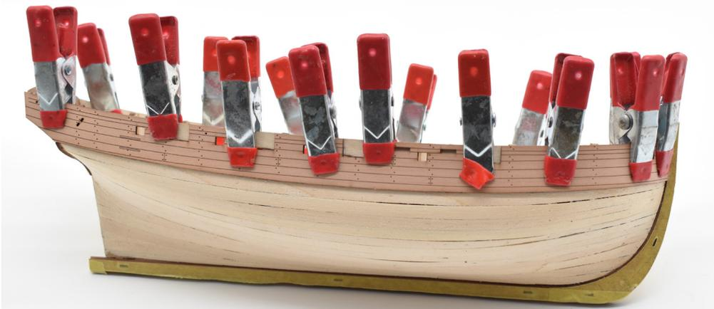
38. Parts 51L and 51R can be either glued into position at this time, or, as we have done here, just clamped into position. I decided to just clamp and not glue these so that I could just get the correct planking line for the 0.8x4mm planking strips, and then remove the engraved outer bulwark before painting the lower hull white, making sure no paint touches the engraved patterns.
