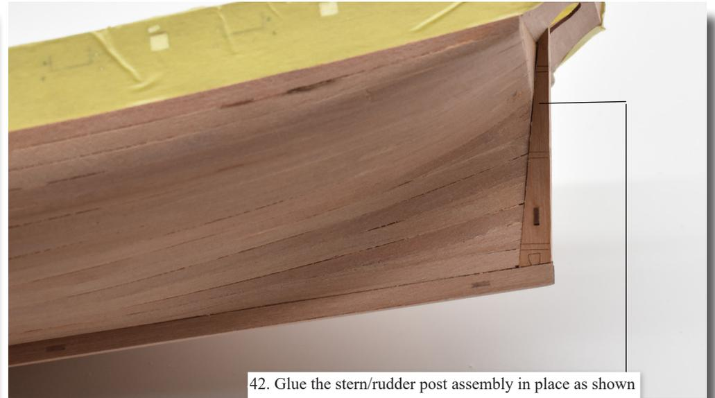
42. Glue the stern/rudder post assembly in place as shown
