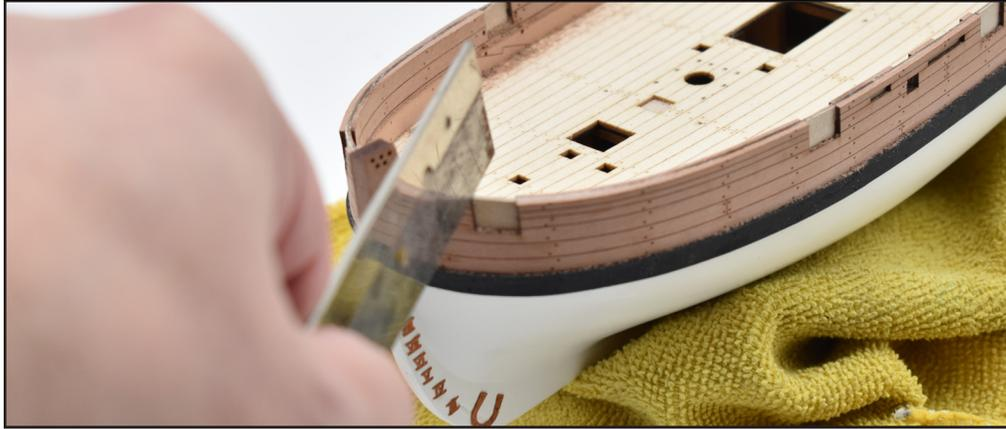
64. Above - using a Razor Saw, carefully cut away the ply gun port openings.
