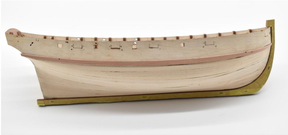
As soon as the first 0.8x4mm plank is placed on both sides, the outer bulwark patterns are removed and kept safe until required later.
