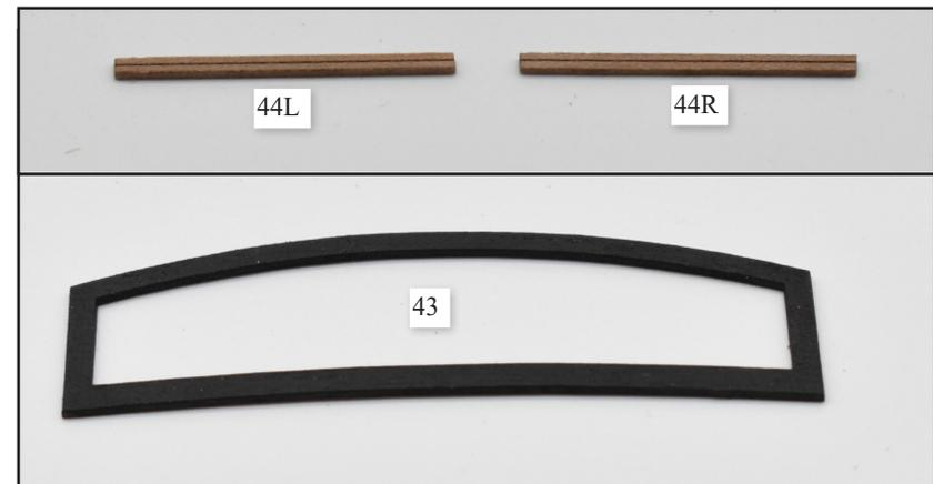
71. Remove the stern transom rail (43) from the 0.8mm wood sheet and paint black. Carefully glue in to its marked position on the stern transom. Remove the stern counter rails (44L and 44R) from the same 0.8mm wood sheet and glue into position as shown in the picture and Plan Sheet 9.
