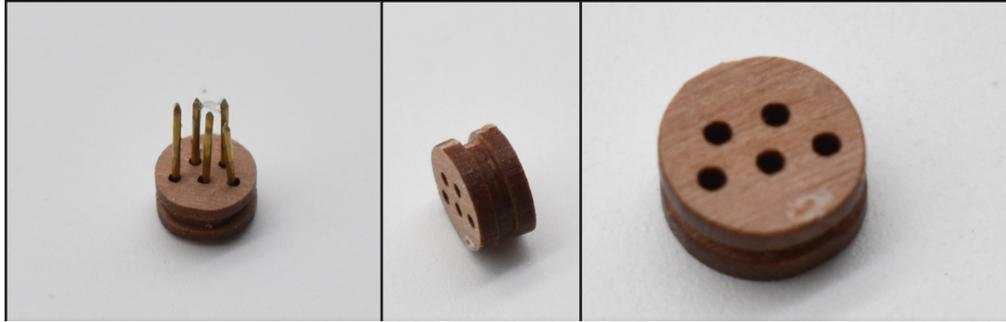
Main Stay 5-Hole Deadeye. Make up this special deadeye as shown using the inner part (77) and the two outer parts (76). These are glued together as shown, but be very careful with the PVA glue, as you do not want to clog any of the five holes. Use pins to both align the three parts and stop any glue from blocking the holes. Remove when the glue has cured.
