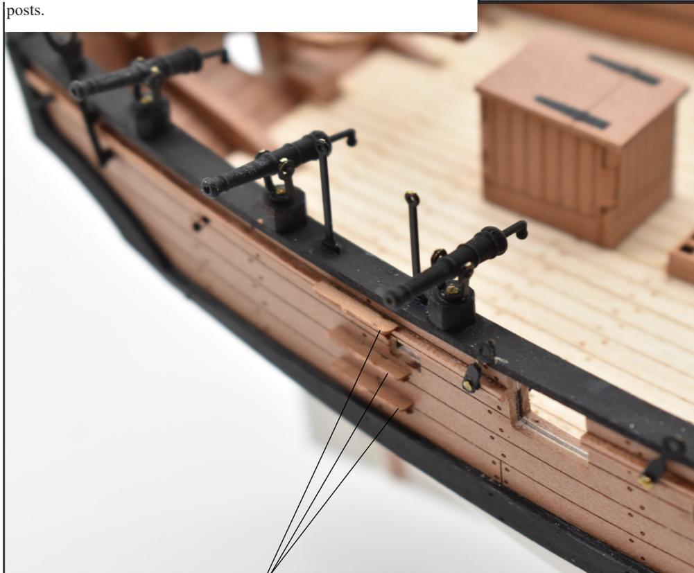
94. The outer hull side steps can now be fitted, These are on the 0.6mm wood sheet, 38 are the lower parts and 39 are the upper parts. The step positions are engraved on the hull sides, so glue in place to these positions using a small amount of PVA wood glue, and tweezers for positioning.
