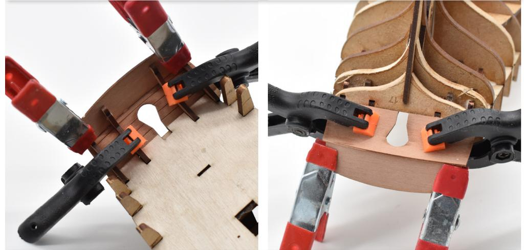
21. Using PVA wood glue, fix and clamp part 62 in place on the four stern frames, the engraved vertical lines lining up with each of the stern frames. Follow this by gluing and clamping the inner stern transom (63). Leave for 24 hours to thoroughly cure.
