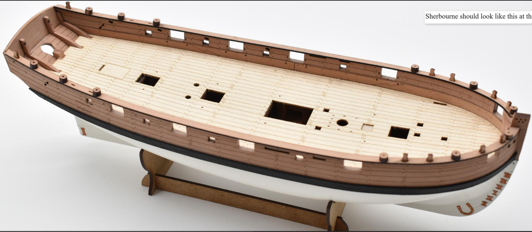
70. Using a spare strip of 0.8x4mm planking strip, cut to size and glue on top of the stern board. Next, paint black and glue the stern side timer (64) as shown. Any slight gaps can be filled with filler, sanded back and repainted.
