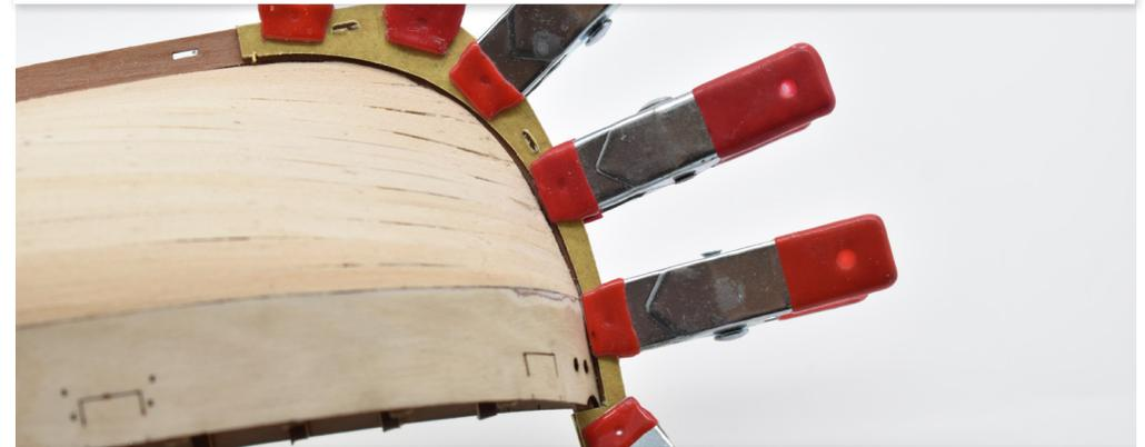
36. Glue the prow patterns in place, using parts 65 for perfect alignment, along with the outer keel sides (58). Use PVA wood glue, but take care to not allow too much glue to seep into the slot for the second planking
