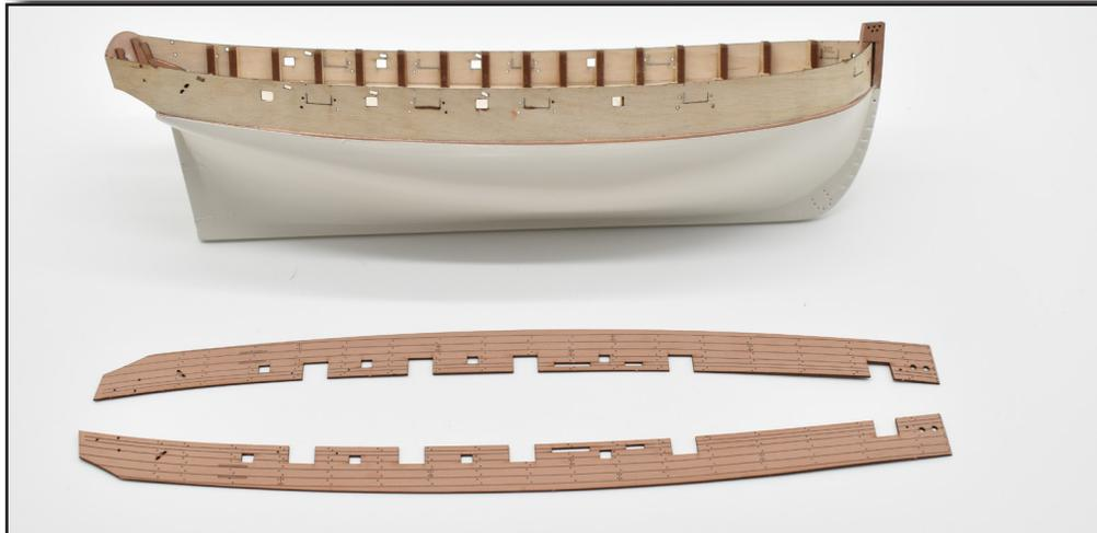
47. Now that all of the 'messy' work has been done, the outer bulwark patterns can now be glued into place. No pins were used, just claps. As with almost all wood to wood fixing, PVA wood glue was used. This was brushed onto the ply side, and the wood engraved bulwark placed and clamped in place, as shown.
