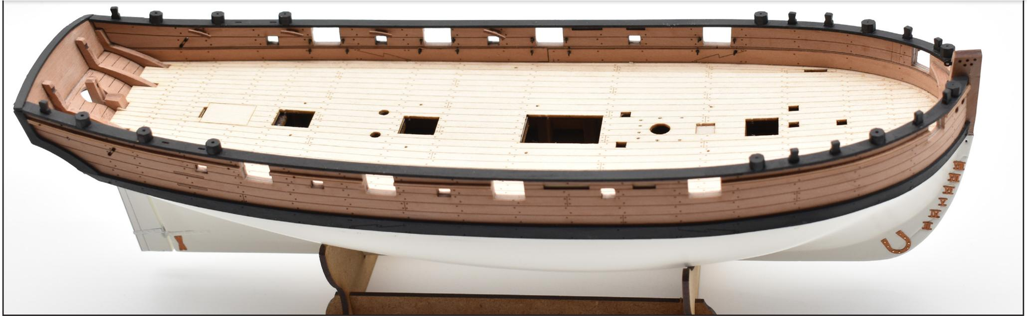
74. Remove the channels (89) from the 1.5mm wood sheet and glue in place. There are slots in the bulwarks so they can only be fitted one way. Use PVA wood glue. Each has a hole for an eyebolt (PE-1), which can also be painted black and glued into the channel at this point,
