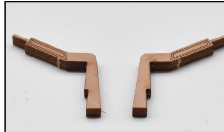
Above - The two halves of the main cathead glued together using PVA wood glue. Right - The sheaves (73) added to the top and bottom ends of the cathead. Below - The cathead assemblies complete, and with the laser char filed off.
