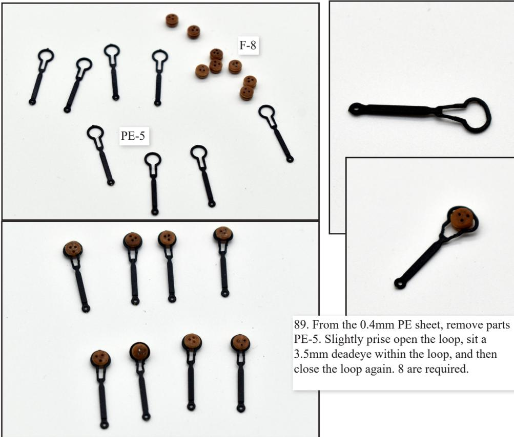
89. From the 0.4mm PE sheet, remove parts PE-5. Slightly prise open the loop, sit a 3.5mm deadeye within the loop, and then close the loop again. 8 are required.
