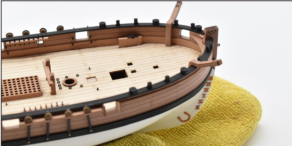
Glue one of the winch side into its slot located on the deck. Also, at this stage, the belaying racks on the bulwark sides have been added, plus deck eyebolts
