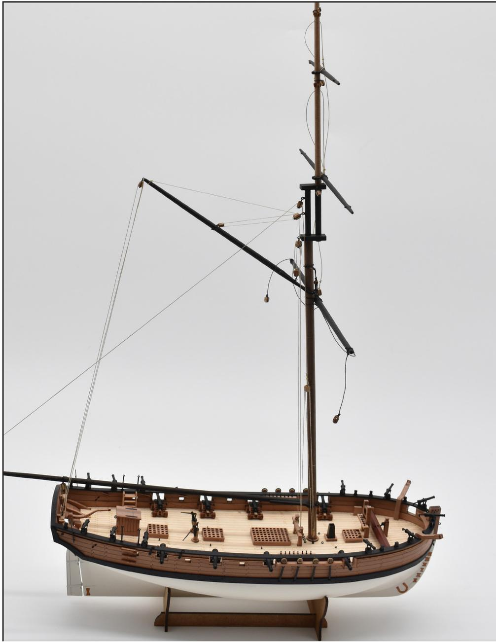
Once the mast assembly is fixed, the boom and gaff yards can be rigged. This should be very easy as there are no other rigging lines to get in the way.
