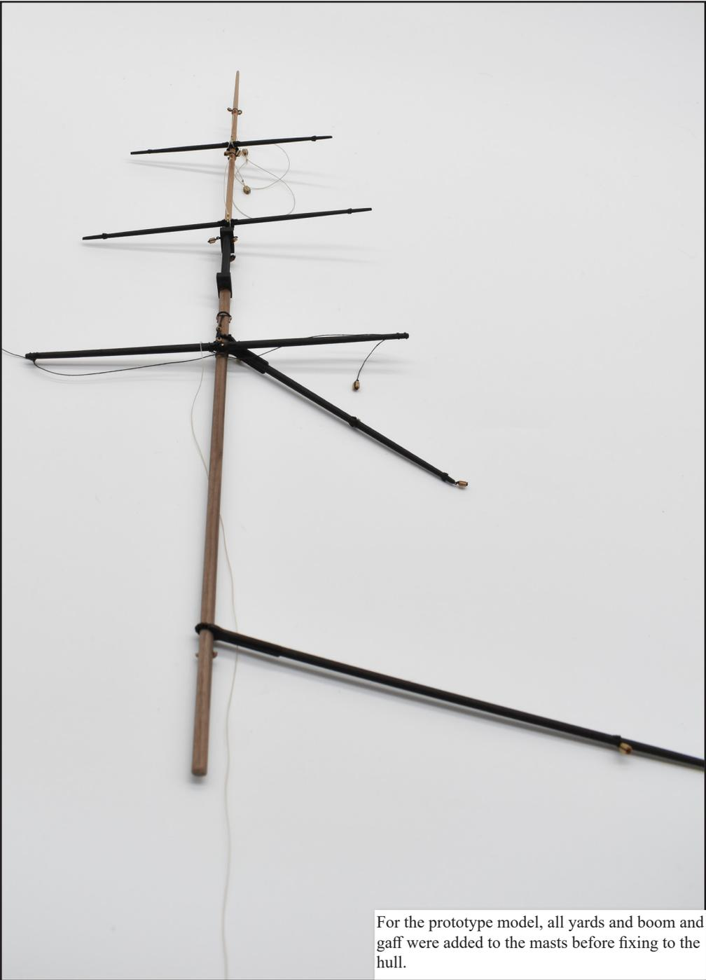
For the prototype model, all yards and boom and gaff were added to the masts before fixing to the hull.
