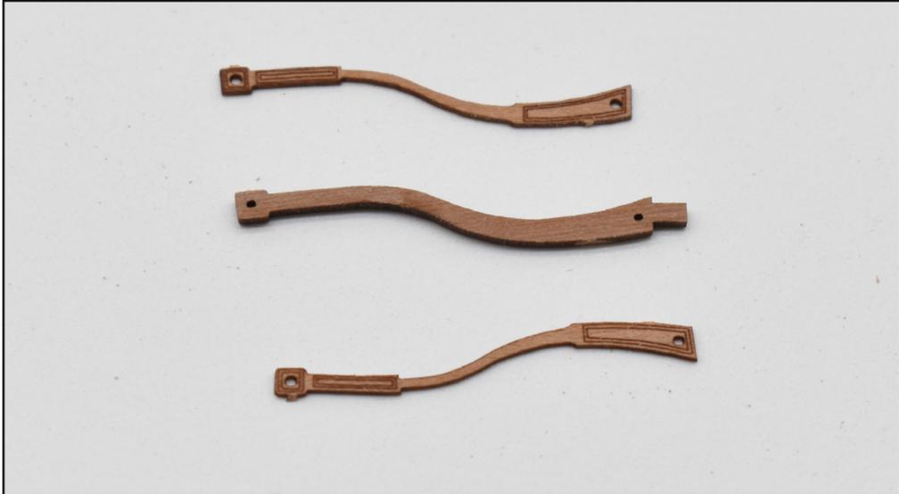
91. Make up the tiller arm with the core (66) the left outer (34L) and right outer (34R). You can use brass pins to help with alignment, and the edges of the tiller arm can be rounded off slightly. Using PVA wood glue, slot the tiller arm into the slot in the rudder head.
